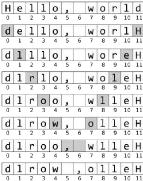
Figure 36-1: The process of reversing a list of single-character strings by swapping their mirror indexes.
